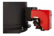
\* Our primary combustion chambers are constructed from high grade steel and monolithic refractory lining with a unique concave design to prevent cold spots. The design ensures a natural secondary burn characteristic as when the burner is switched on a flame curtain is created, this ensures the thermal breakdown of smoke/emissions, where in many instances emissions will exit through the stack and into the atmosphere in the form of clean vapor.
